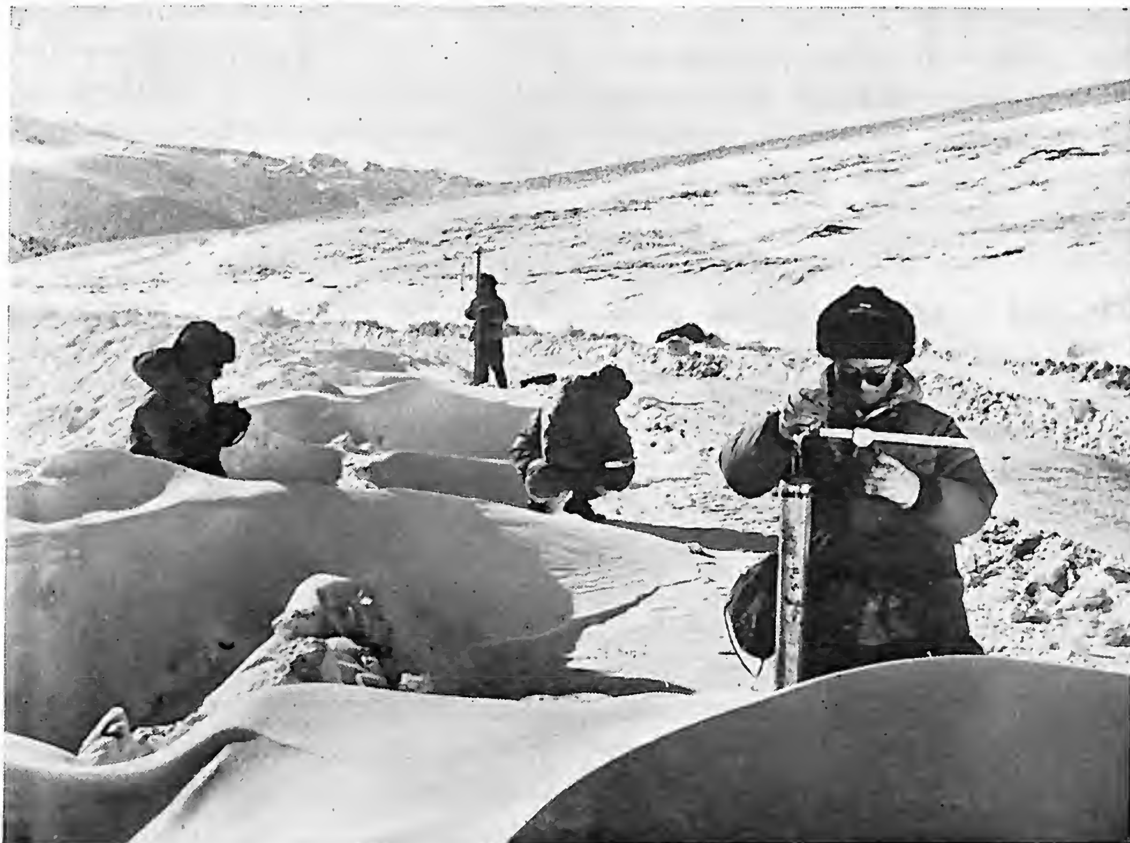
Weighing a snow core to determine density of snow in a drift.
